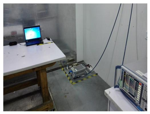
FCC RADIATED EMISSION TEST SETUP
