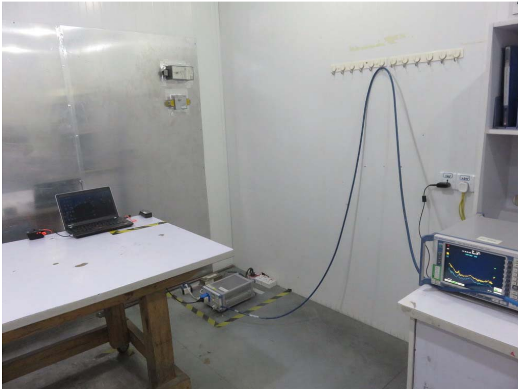
FCC RADIATED EMISSION TEST SETUP
