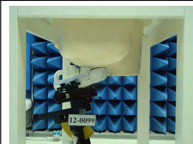
Figure 5. Left Head SAR Test Setup (Tilted)
