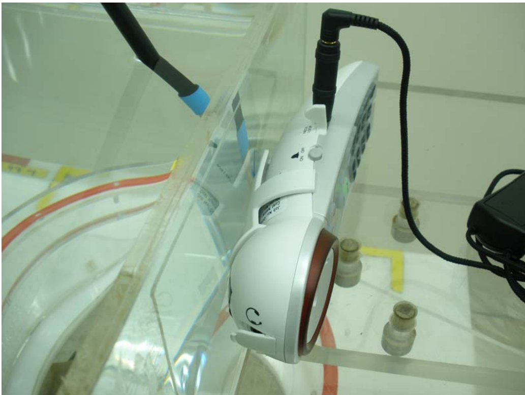
EUT rear to phantom, belt-clip separation with neckloop – Zoom In
