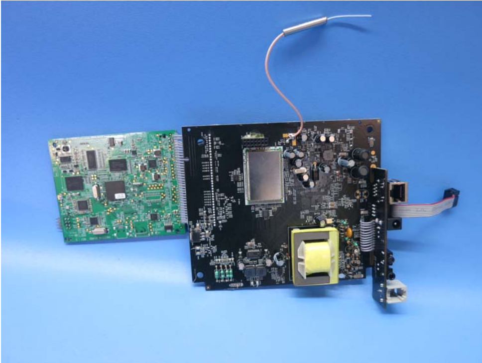
Base Unit – DECT Antenna
