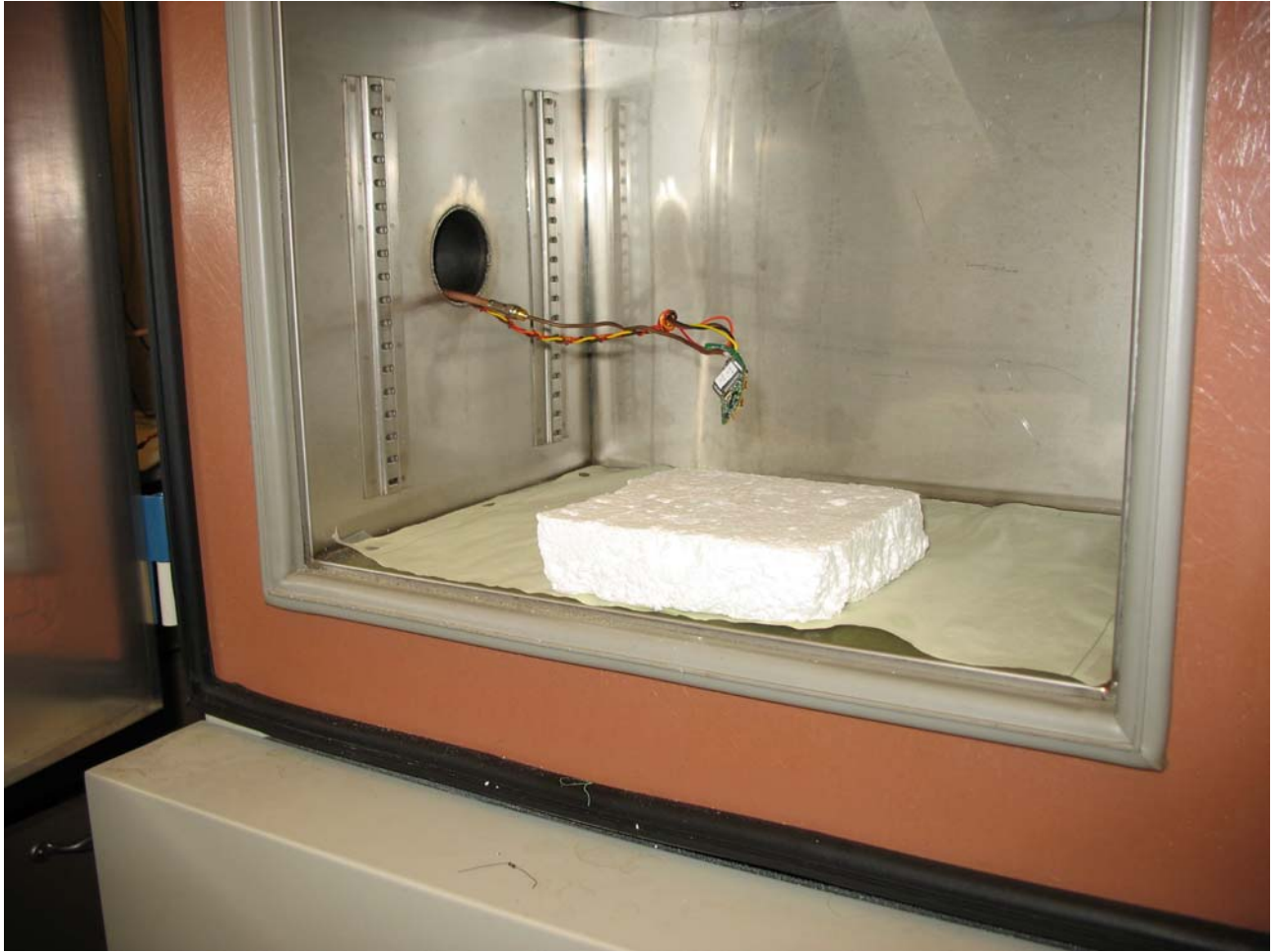
Fig. 38 - Headset EUT within the temperature chamber, with RF connection to EUT and with power/control cable connection to EUT.
