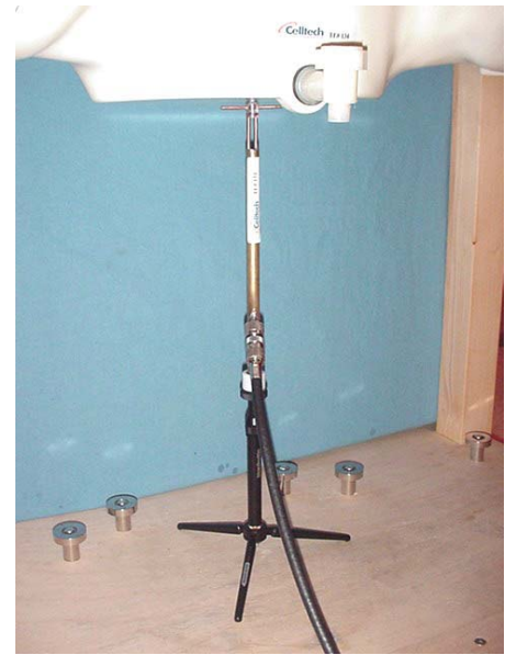
1900MHz Dipole Setup
