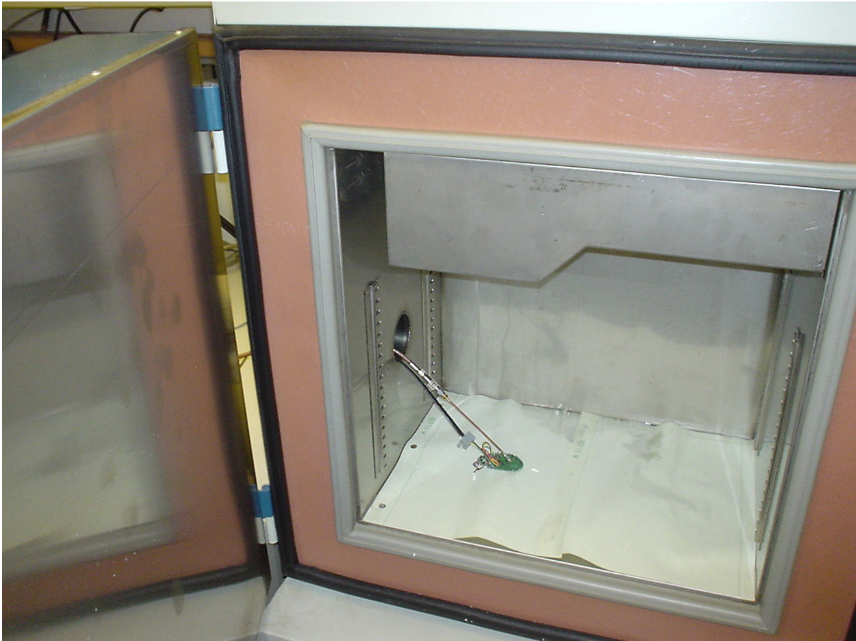
Fig. 111 - Headset EUT within the temperature chamber, with RF connection to EUT and with power/control cable connection to EUT.
