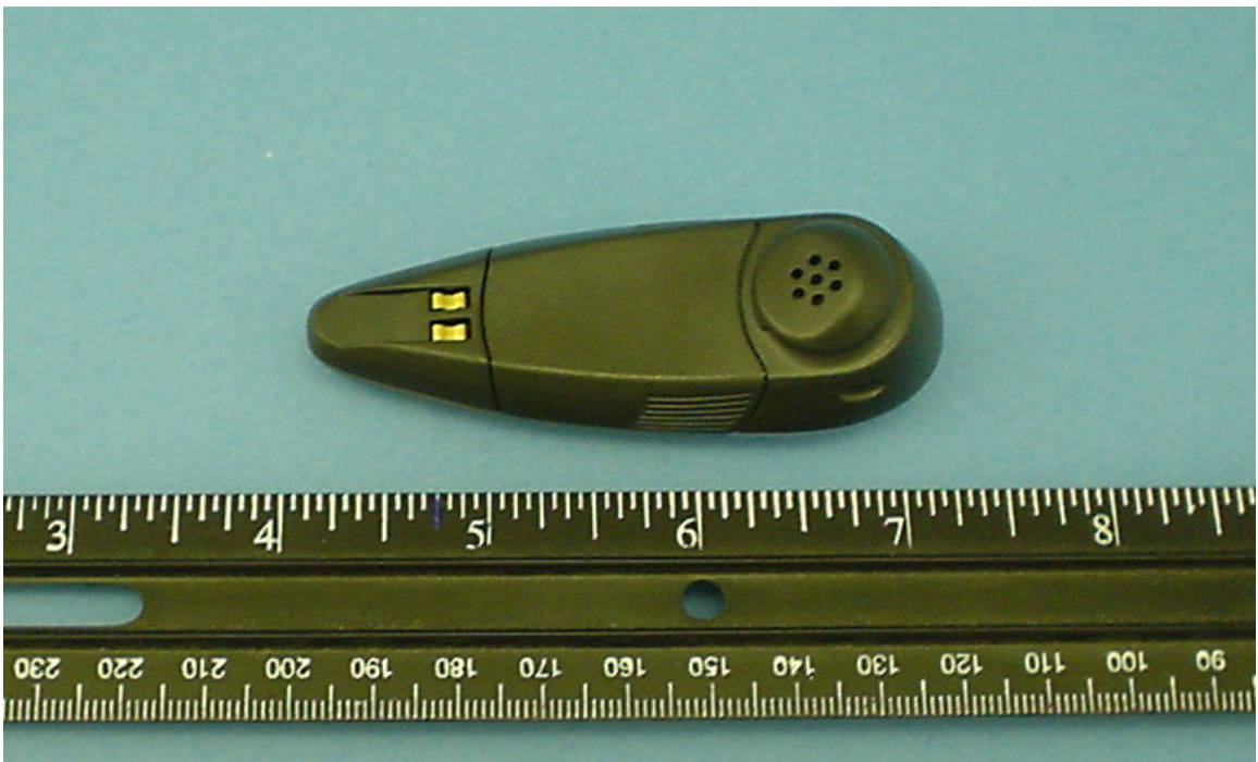
AL8CS55YYYY, reverse side, unit with microphone mounted in short-mount position
