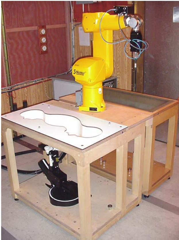
DASY4 Measurement System with SAM Phantom
