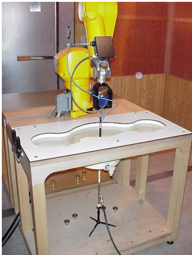
DASY4 Measurement System with SAM Phantom
