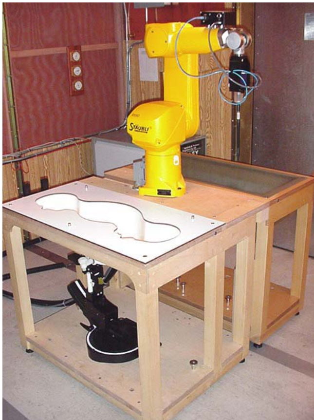
DASY4 SAR Measurement System with SAM Phantom
