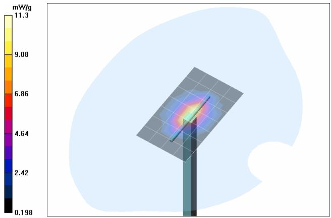
1 g average of 10 measurements: 9.972 mW/g 10 g average of 10 measurements: 5.191 mW/g
