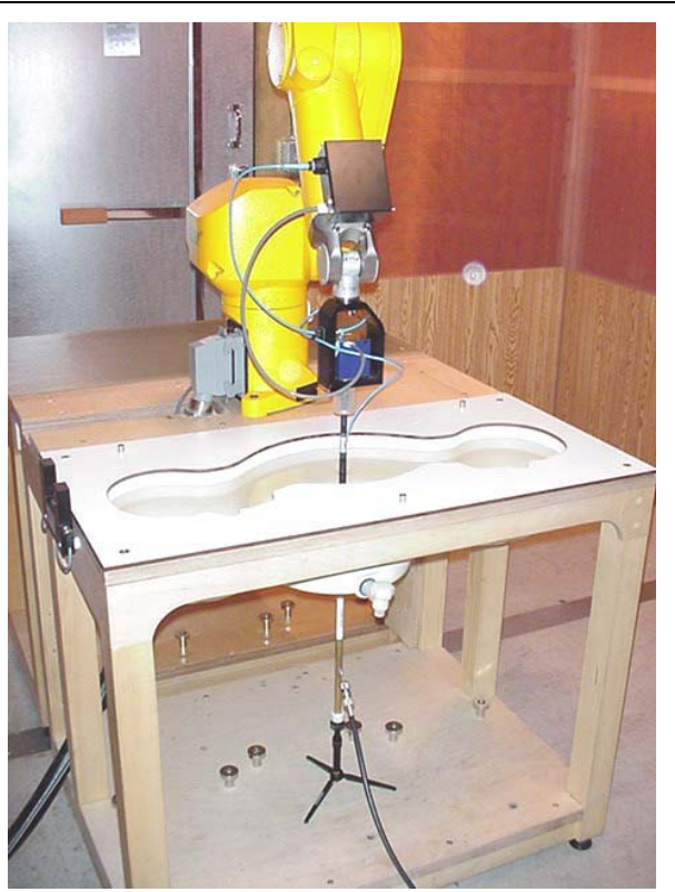
DASY4 Measurement System with SAM Phantom and validation dipole
