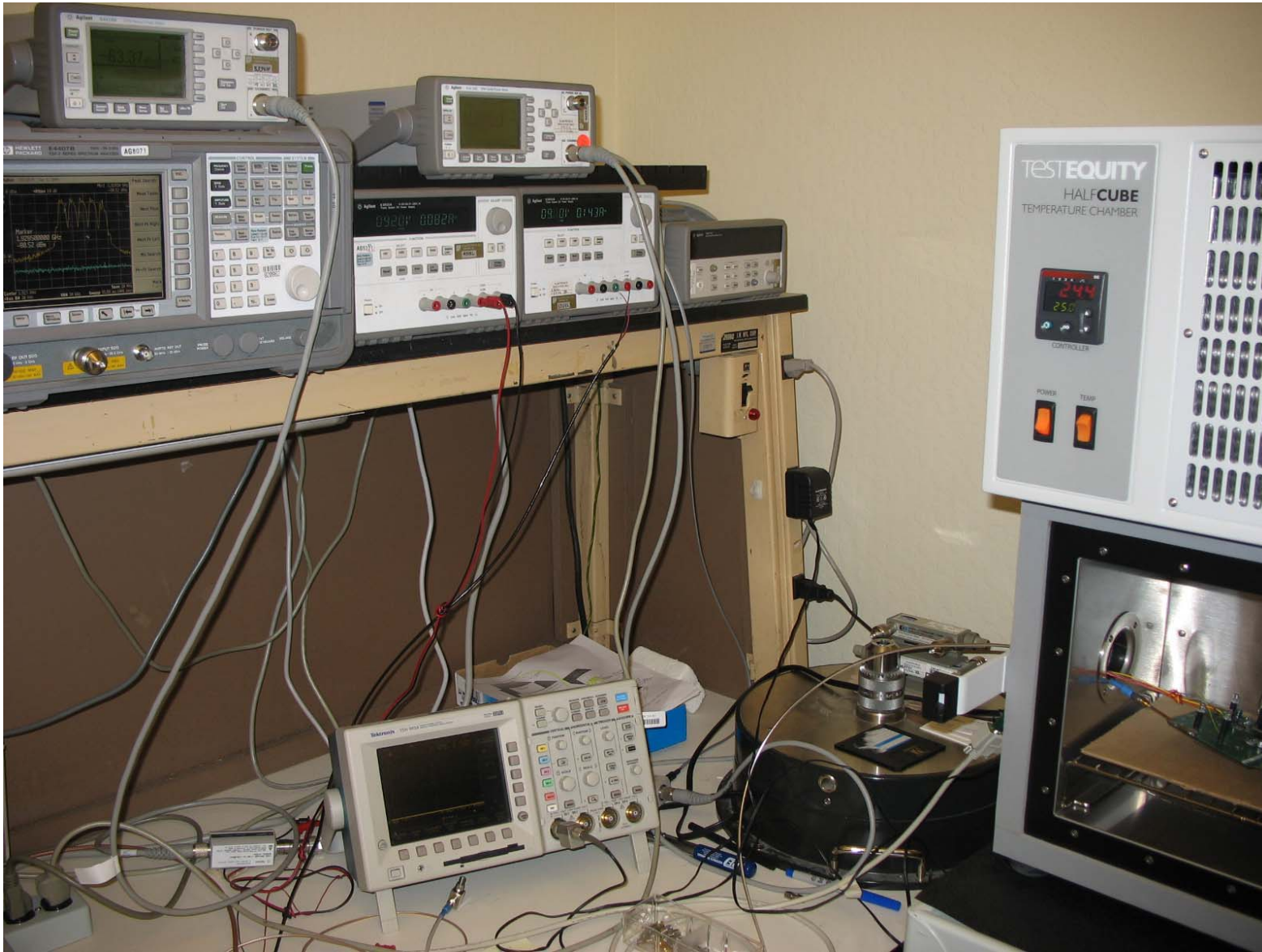
Fig. 41 - View of test system configured for the tests of clause 6.2.1 for the base EUT. EUT is in the temperature chamber at right. EUT power supply is top right-center. EUT RF cabling is connected as described in the text, to the CMD60 analyzer and the E4407B spectrum analyzer. The controller interface circuit (RS232 to CMOS levels) is directly outside the chamber egress.
