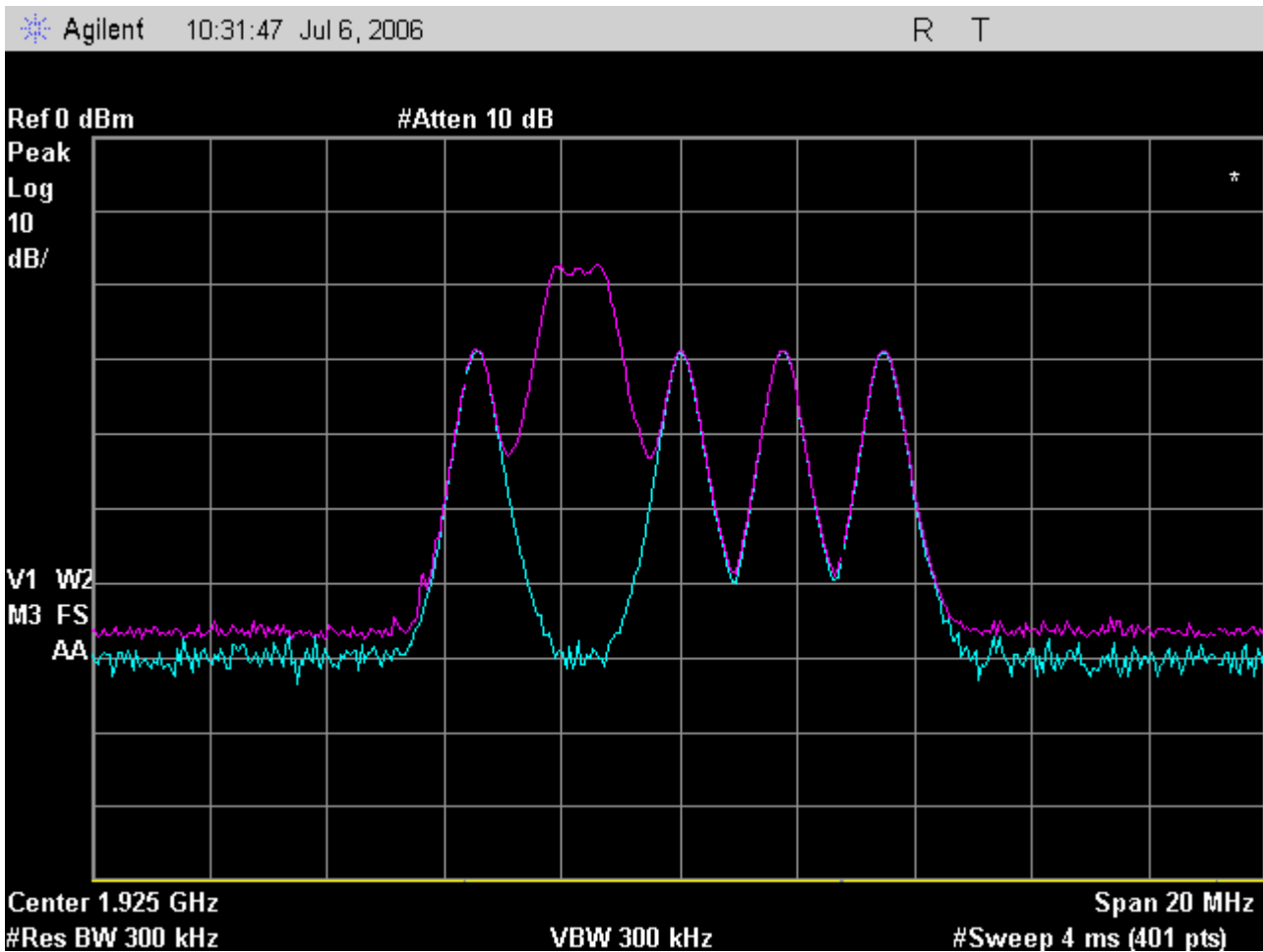
Fig. 56 - Spectrum showing initial interference profile, and transmissions on un-interfered carrier frequency f_2 , for 7.3.4(b)
