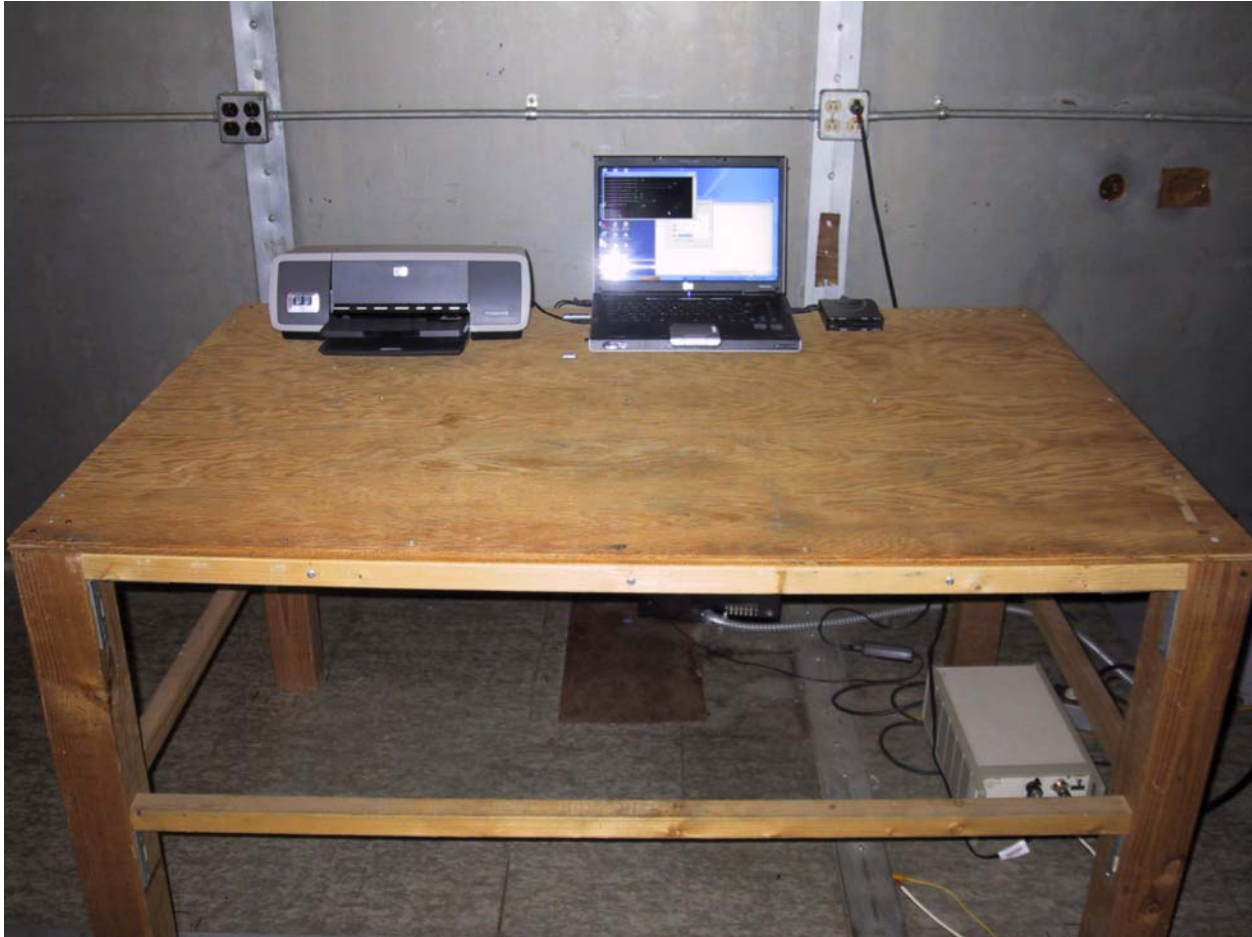
Line Conducted Emissions Test Setup
