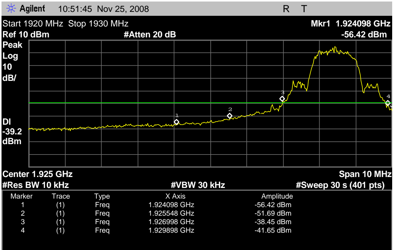
Fig. 22 - Spectrum analyzer screenshot for transmit emissions showing in-band unwanted emissions with the Base EUT transmitter at the highest carrier, 1928.448MHz, according to the requirements of 6.1.6.1.
