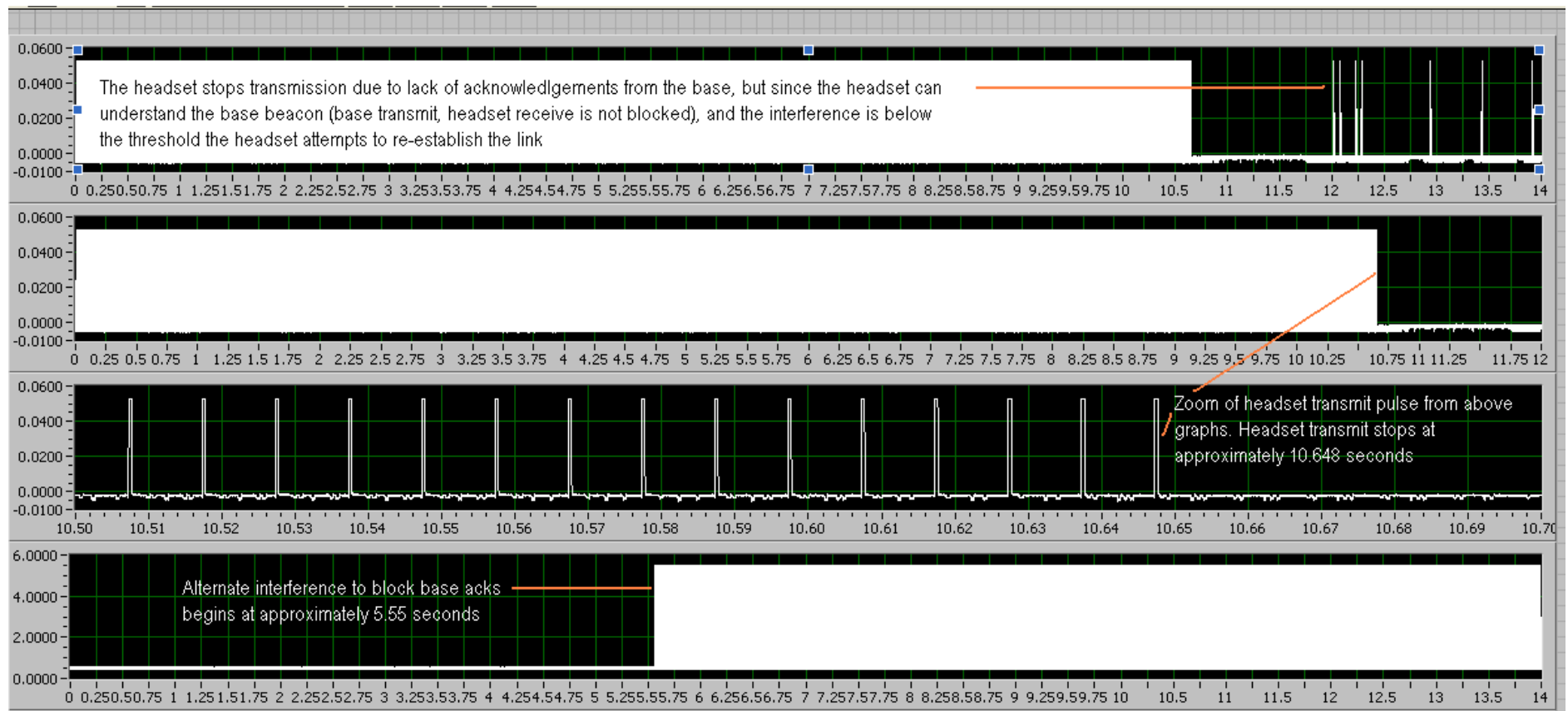
Fig. 66 - RF detector (top three traces) and alternate interference output (bottom trace) as headset EUT transmission goes blocked and transmissions stop.
