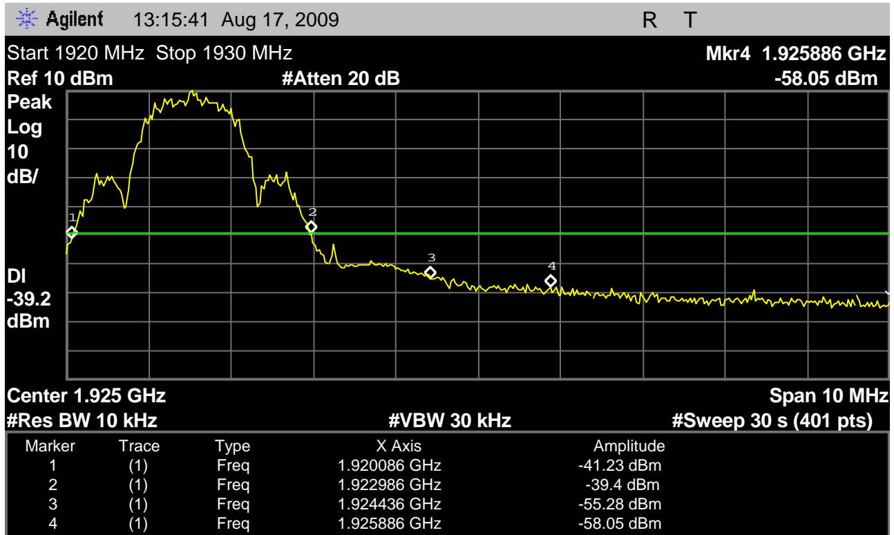
Fig. 20 - Spectrum analyzer screenshot for transmit emissions showing inband unwanted emissions with the headset EUT transmitter at the lowest carrier, 1921.536MHz, according to the requirements of 6.1.6.1.
