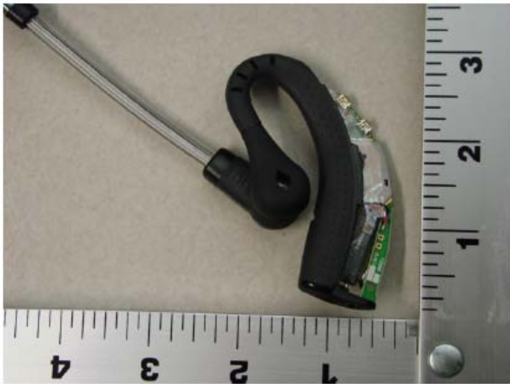
PCB Installed in Headset Left.
