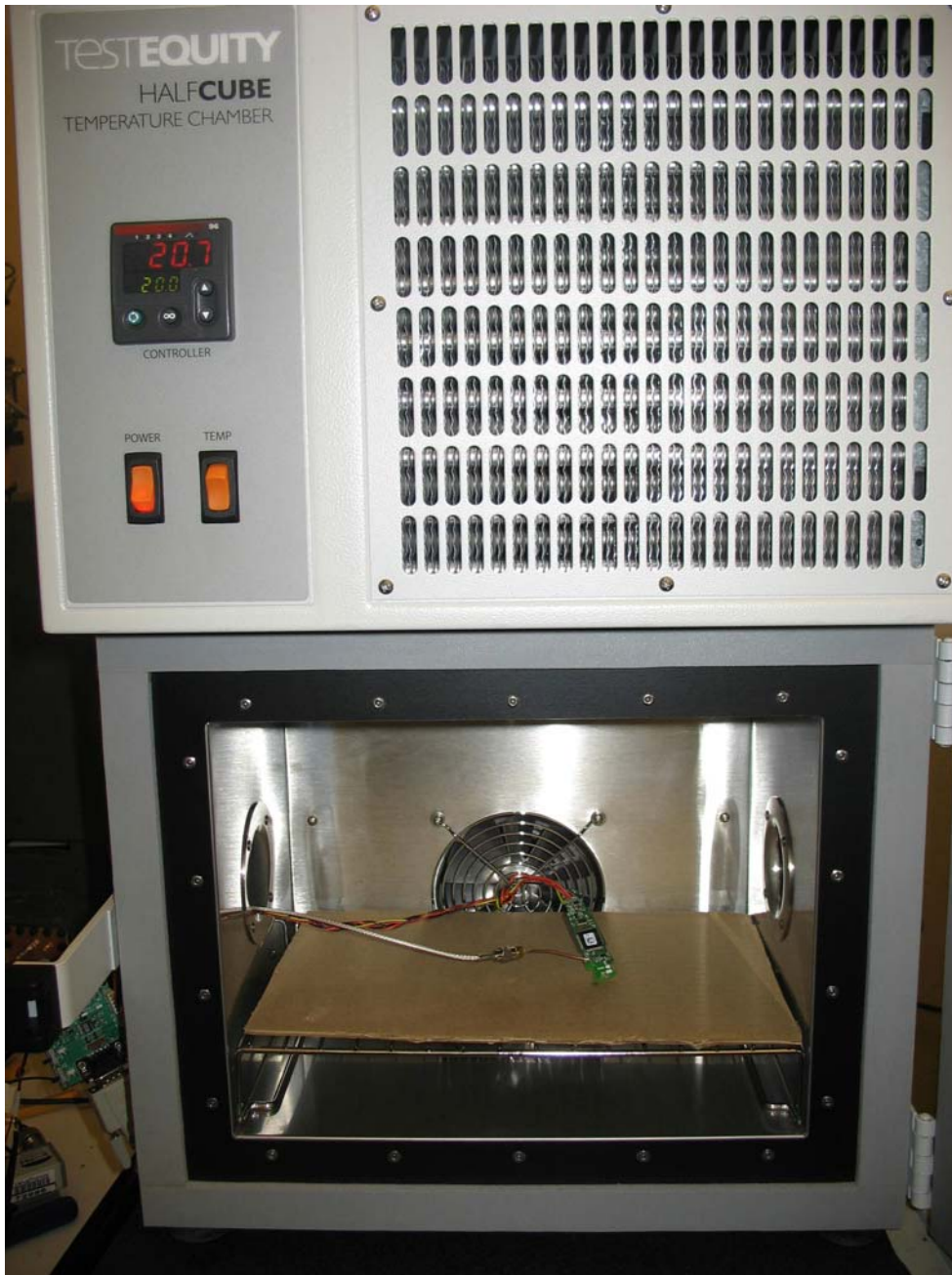
Fig. 39 - Headset EUT within the temperature chamber, with RF connection to EUT and with power/control cable connection to EUT.
