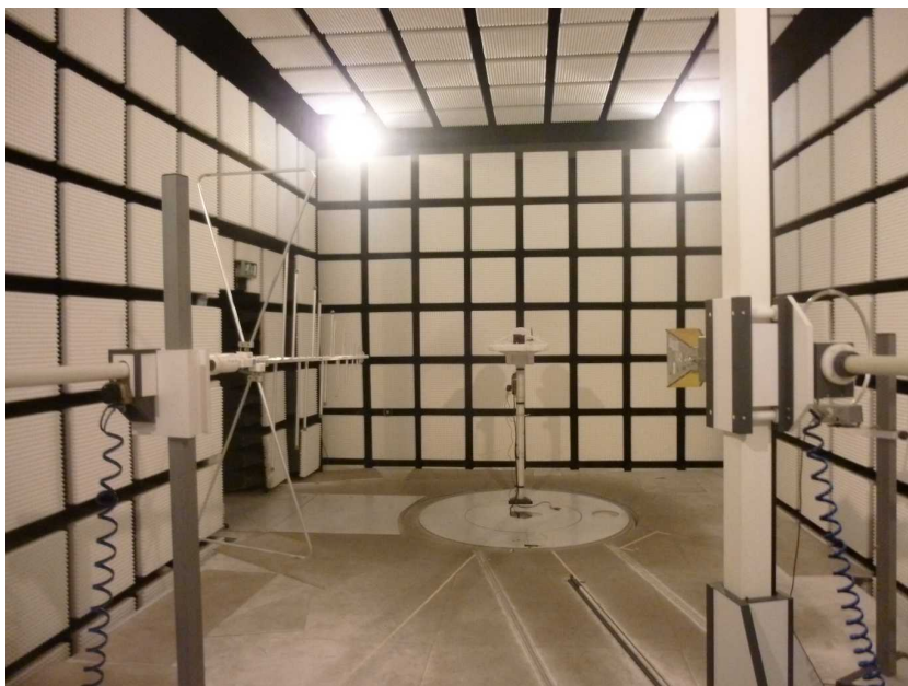
Photo 6: EUT at the anechoic chamber
