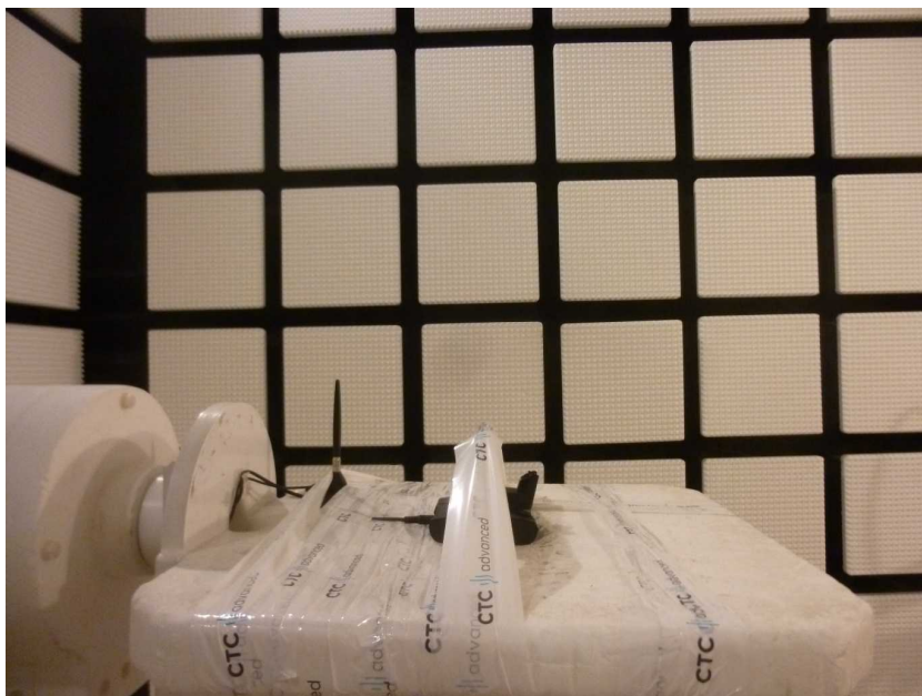
Photo 4: EUT at the anechoic chamber
