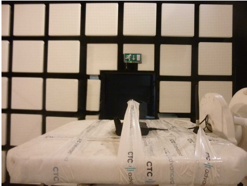
Photo 3: EUT at the anechoic chamber
