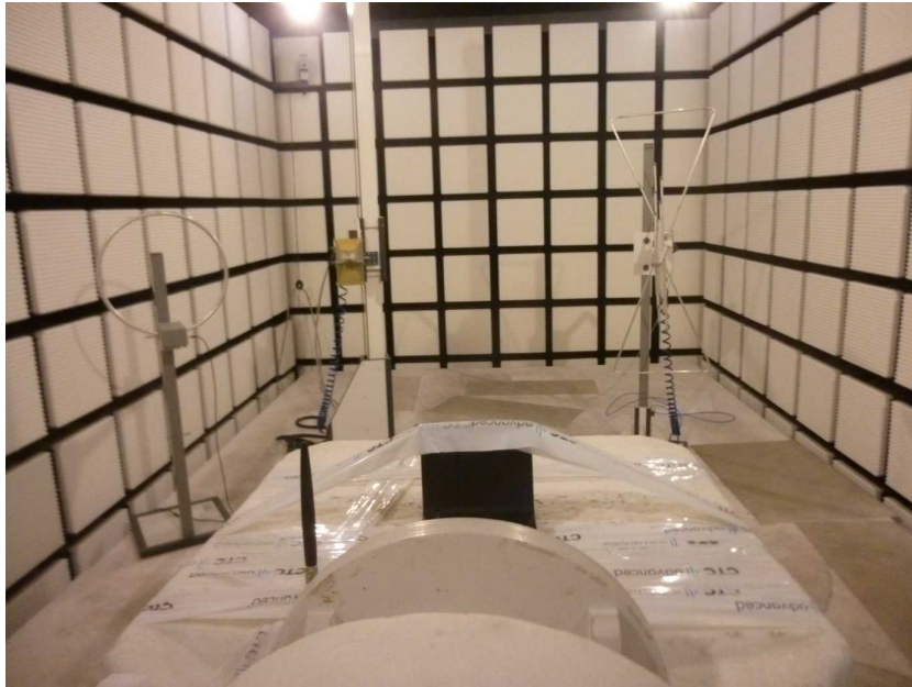
Photo 5: EUT at the anechoic chamber
