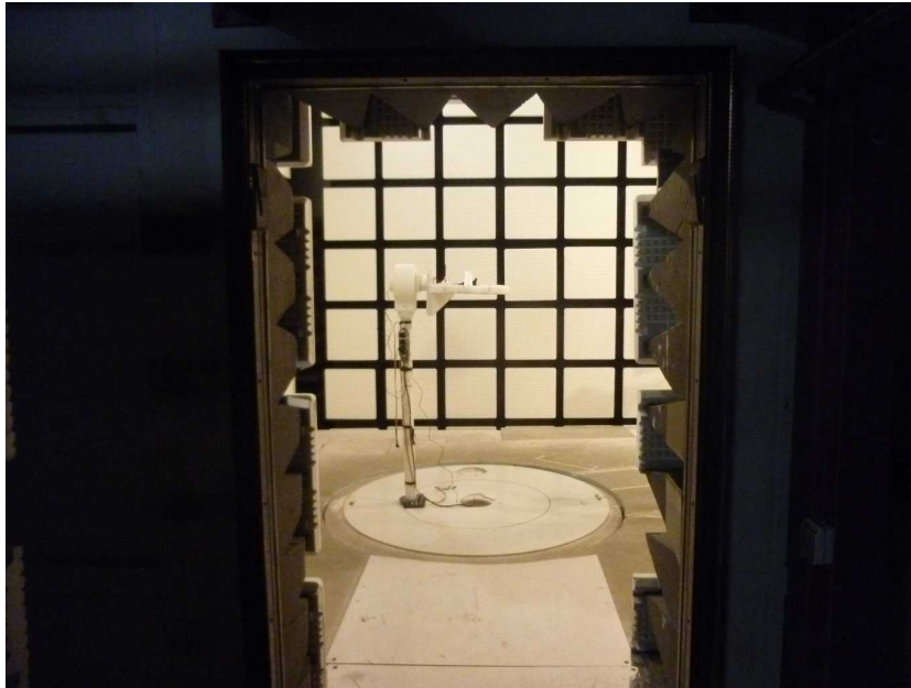
Photo 1: EUT at the anechoic chamber
