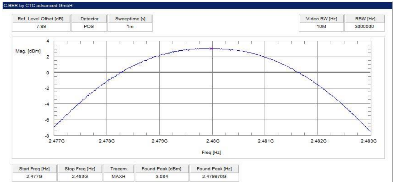
Plot 6: highest channel – 2480 MHz, Pi / DQPSK modulation
