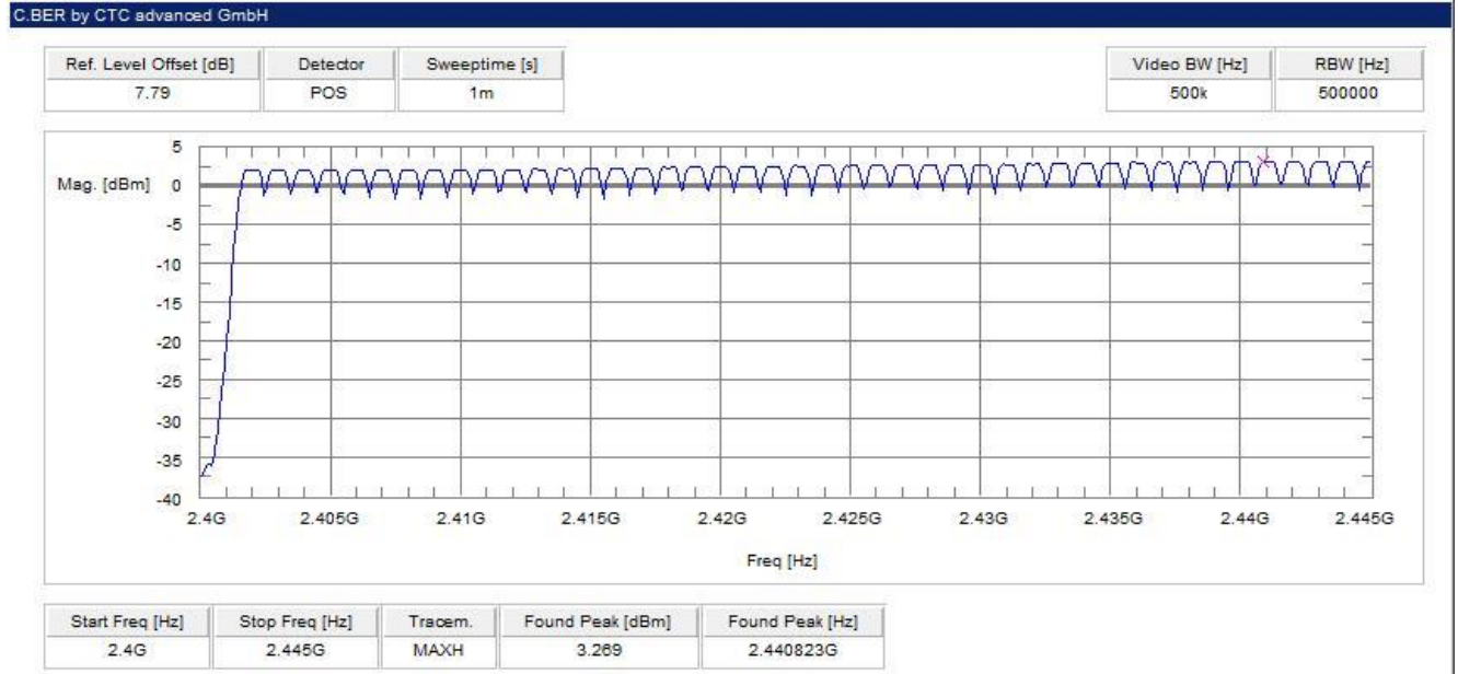
Plot 1: Number of hopping channels (GFSK modulation)
