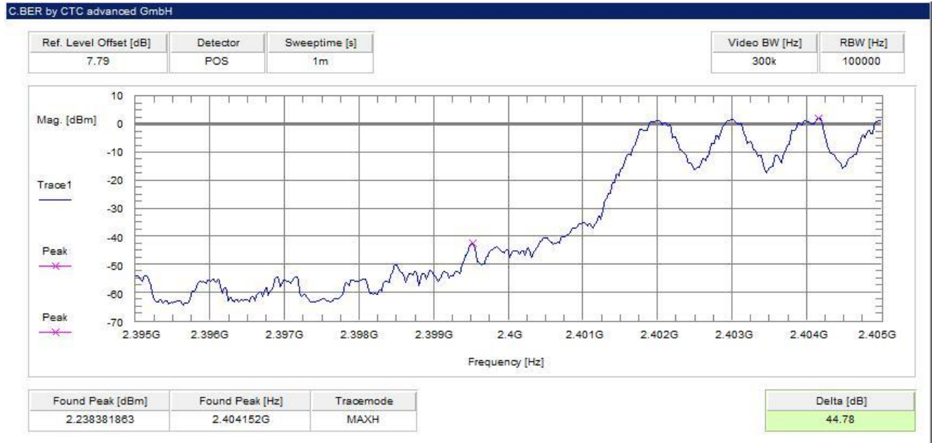
Plot 1: Lower band edge – hopping on, GFSK modulation
