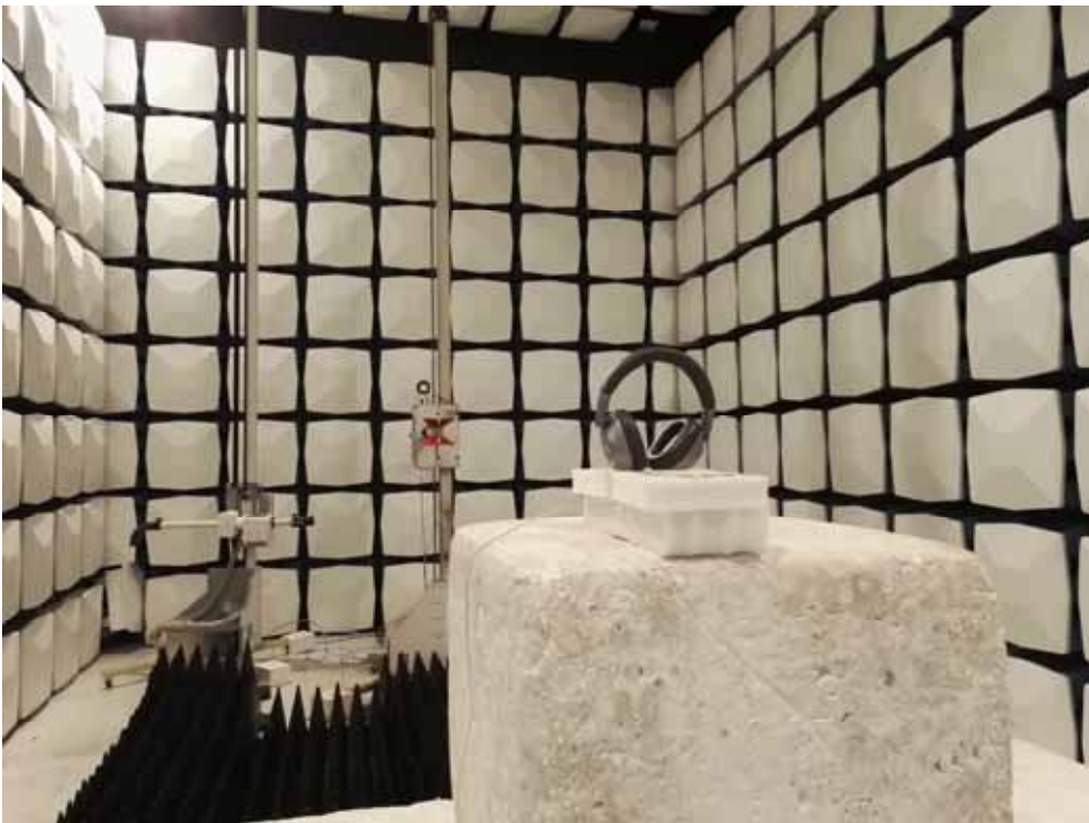
Description: Radiated Emission Test Setup for 1~18GHz
