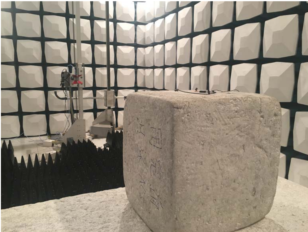
Description: Radiated Emission Test Setup for 1~18GHz
