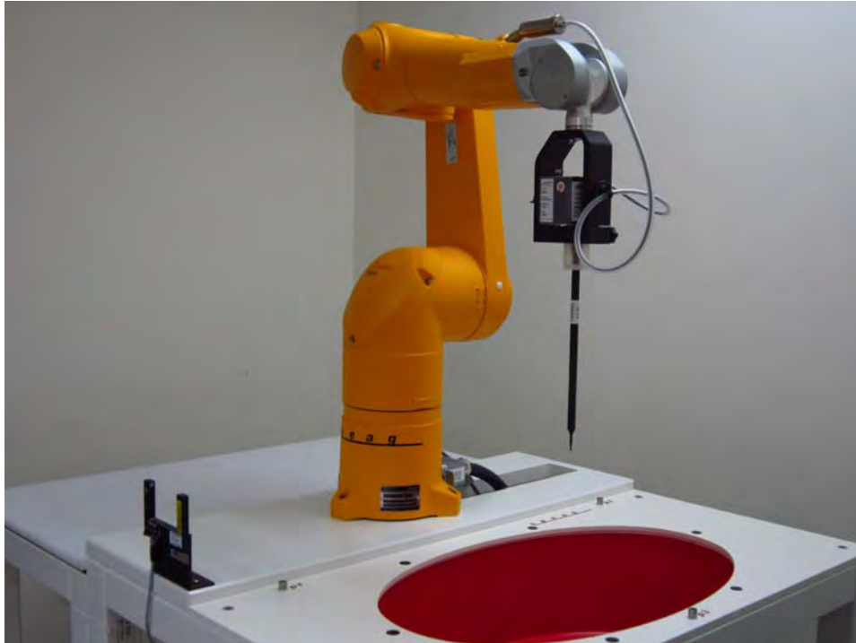
Fig.1 Photograph of the SAR measurement system
