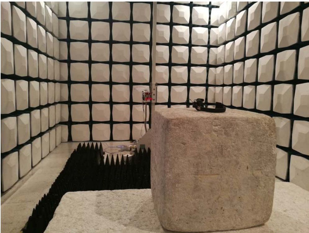
Description: Radiated Emission Test Setup for 1~18GHz
