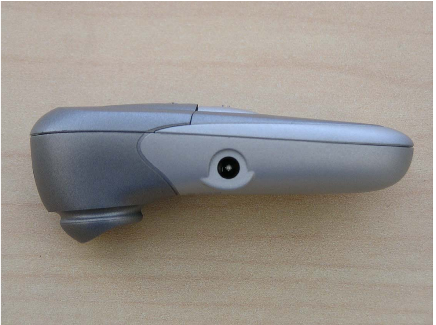
EUT – Profile view showing DC power port
