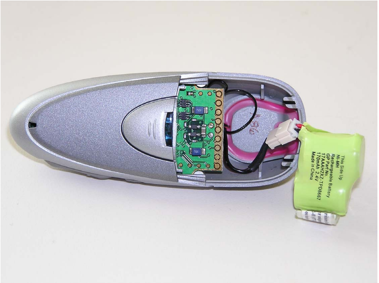
EUT – Open view showing battery
