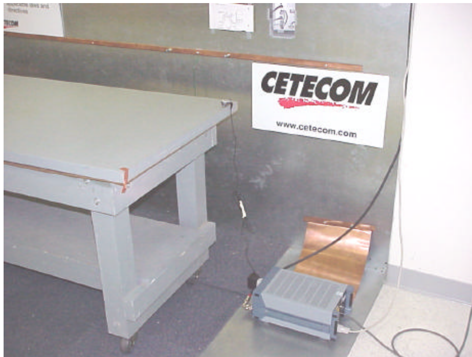
Test setup – AC Line conducted emissions
