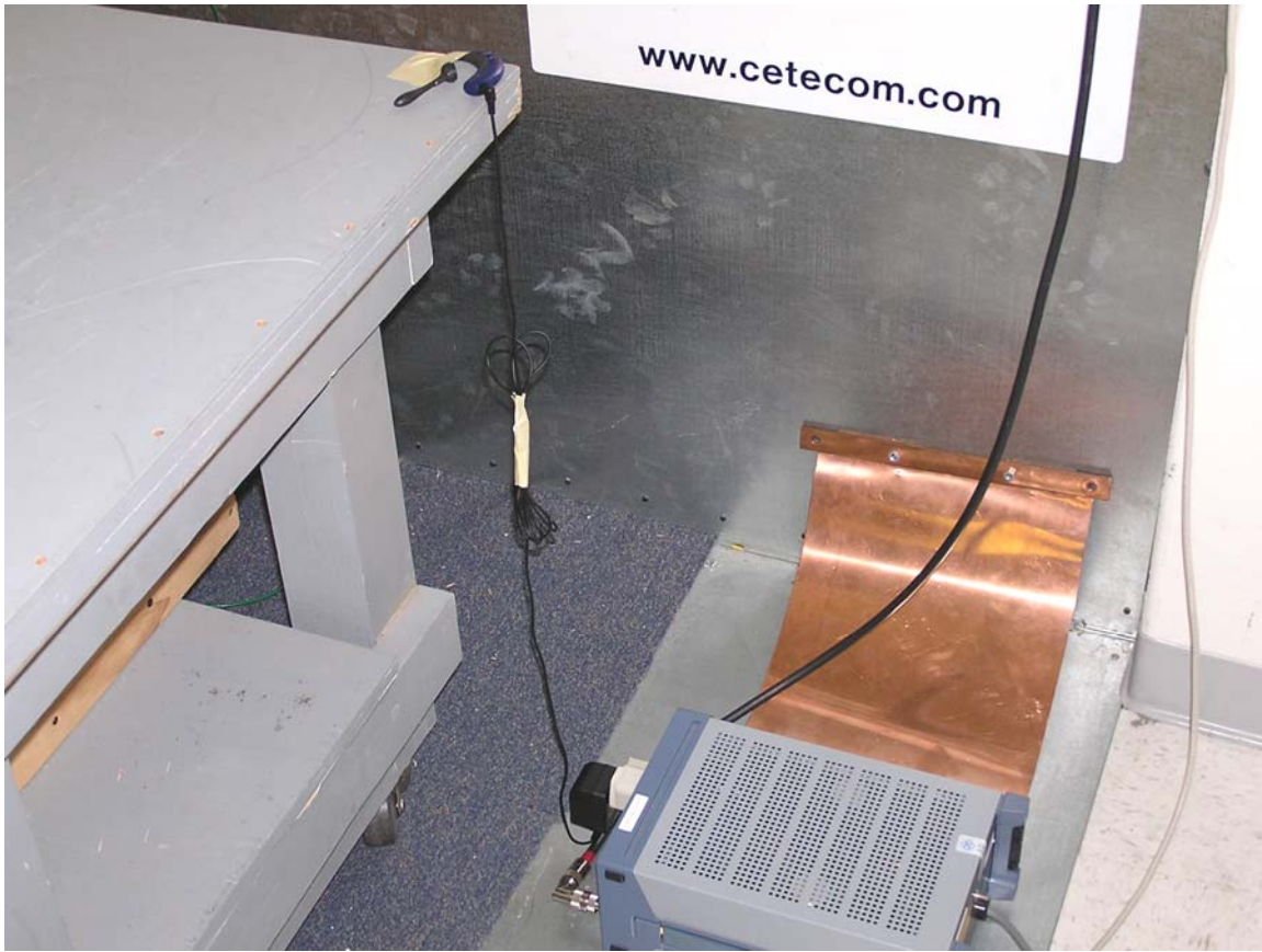
Test setup – AC Line Conducted Emissions
