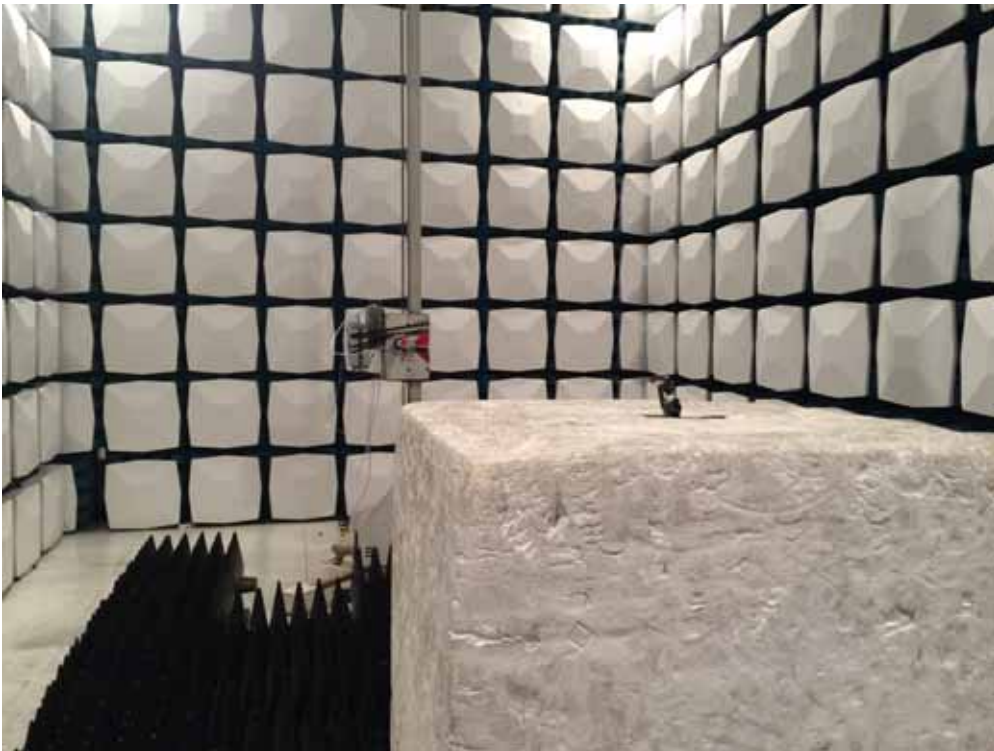
Description: Radiated Emission Test Setup for 1~18GHz
