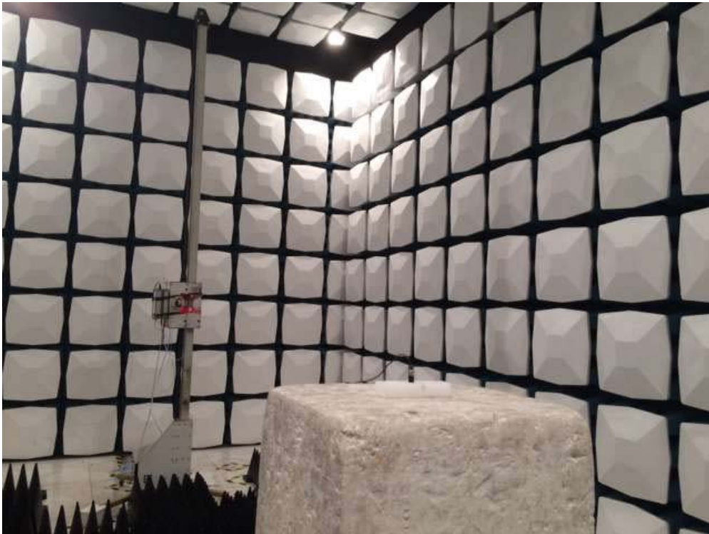
Description: Radiated Emission Test Setup for 1~18GHz
