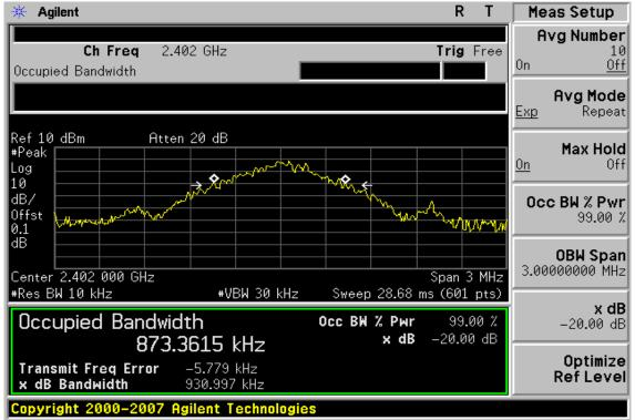
20dB Bandwidth Test Data CH-Mid
