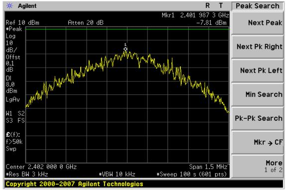
Power Spectral Density Test Plot (CH-Mid)
