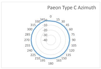
Azimuth Peak Gain .063dBi
