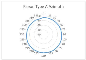
Azimuth Peak Gain -.053 dBi
