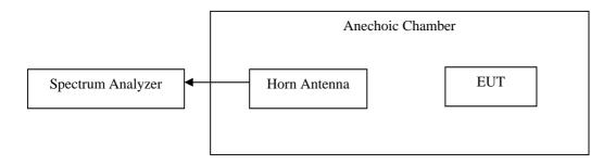
This setup is used for measuring the radiated output power in a fully anechoic chamber with a measurement distance of 1m.
