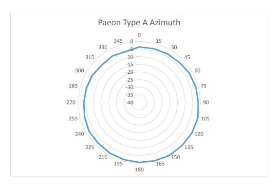
Azimuth Peak Gain -.053 dBi
