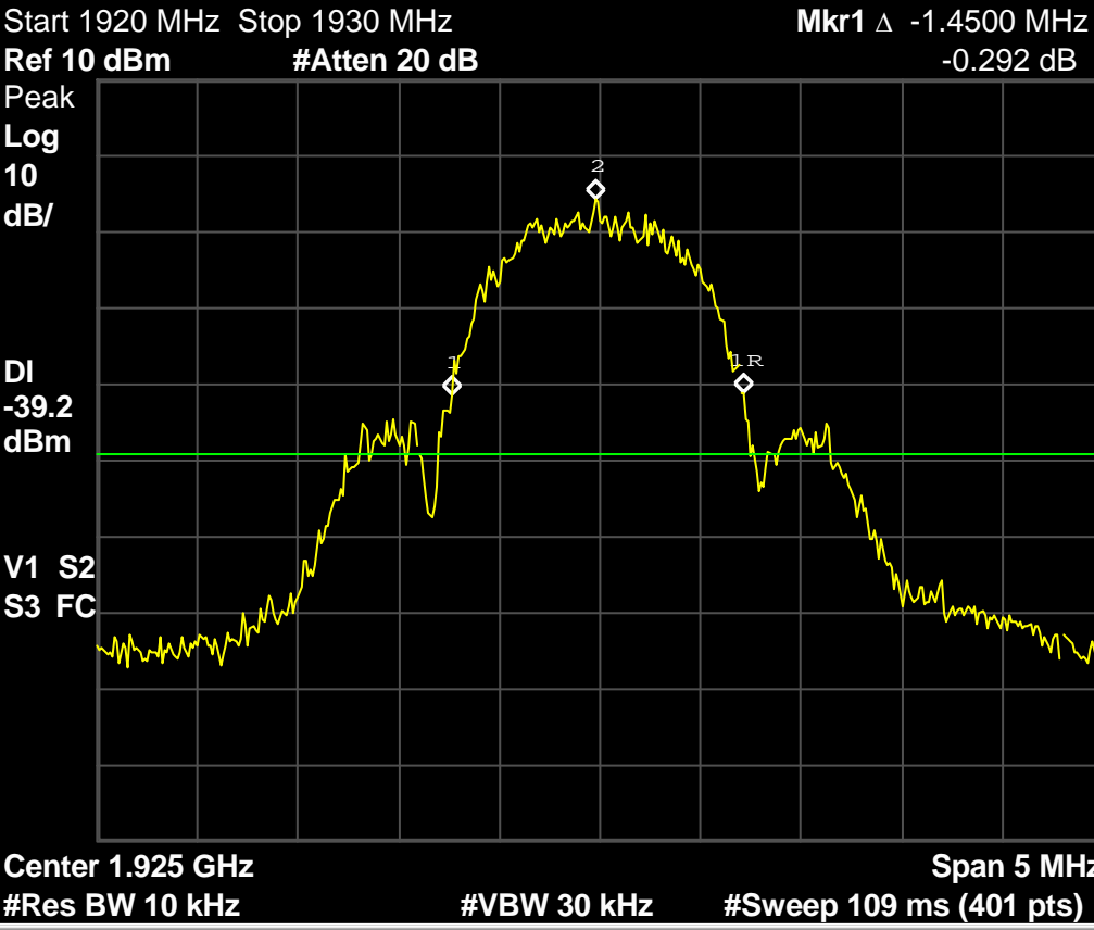
Fig. 68 - Base EUT in low power WBM, 1.45MHz emissions bandwidth on mid carrier vs. 1.42MHz in max power normal mode.
