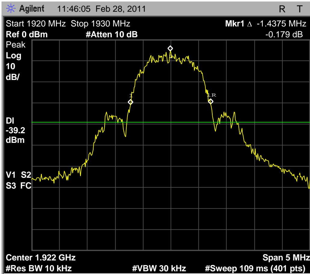
Fig. 67 - Base EUT in low power WBM, 1.4375MHz emissions bandwidth on low carrier; vs. 1.435MHz in max power normal mode.
