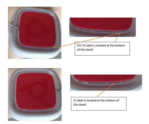
The regulatory markings/nameplate data are legibly printed on a 0.8mm thick PET film with 0.08mm thick pressure sensitive adhesive, the label is affixed on the bottom enclosure which is a permanently attached part of the charge stand. The label is visible, but not touchable to user, this ensure the label is visible and indelible.
