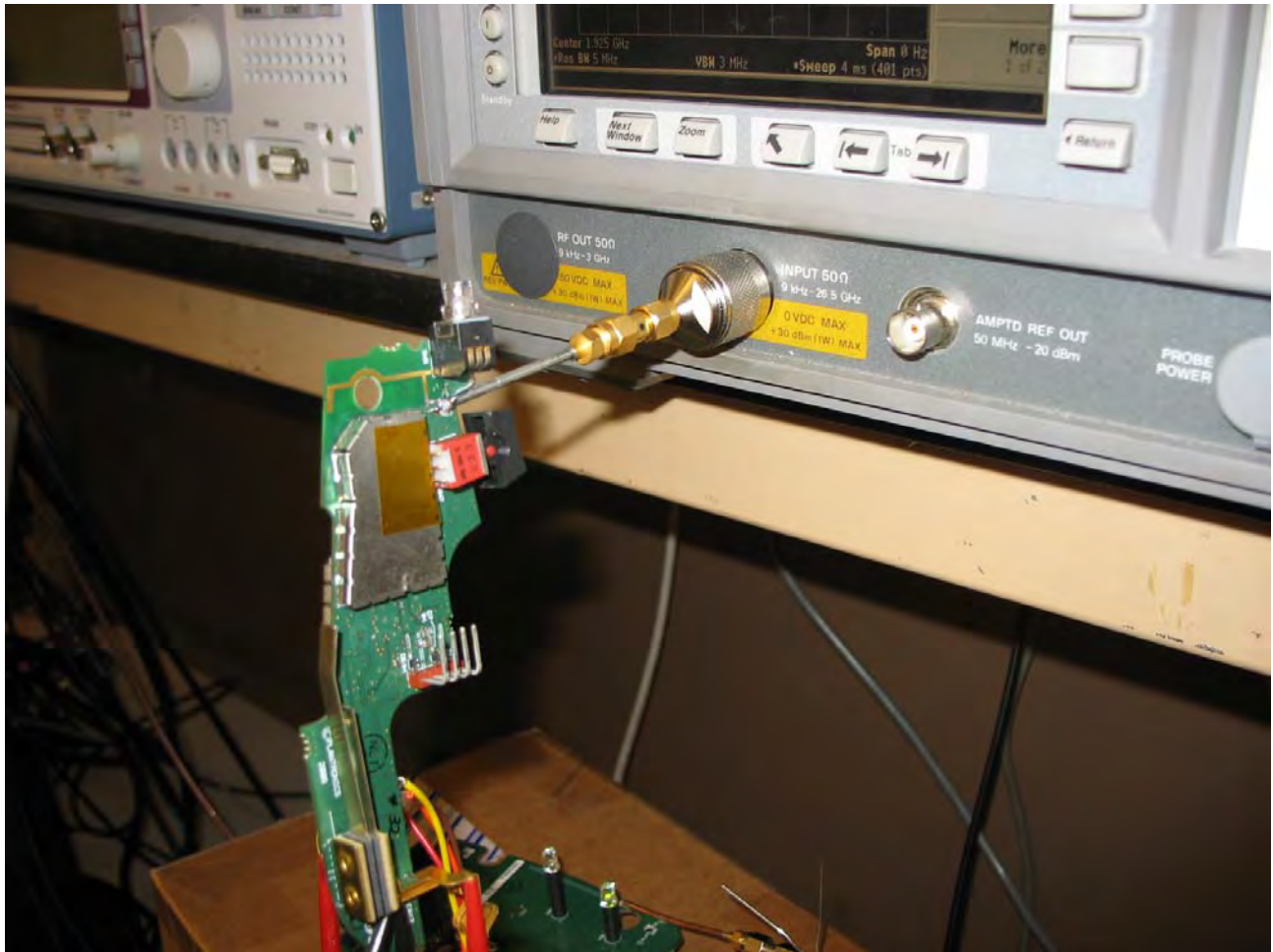
Fig. 79 – Remote EUT- Detail of the attachment of the RF connection for conducted measurements.
