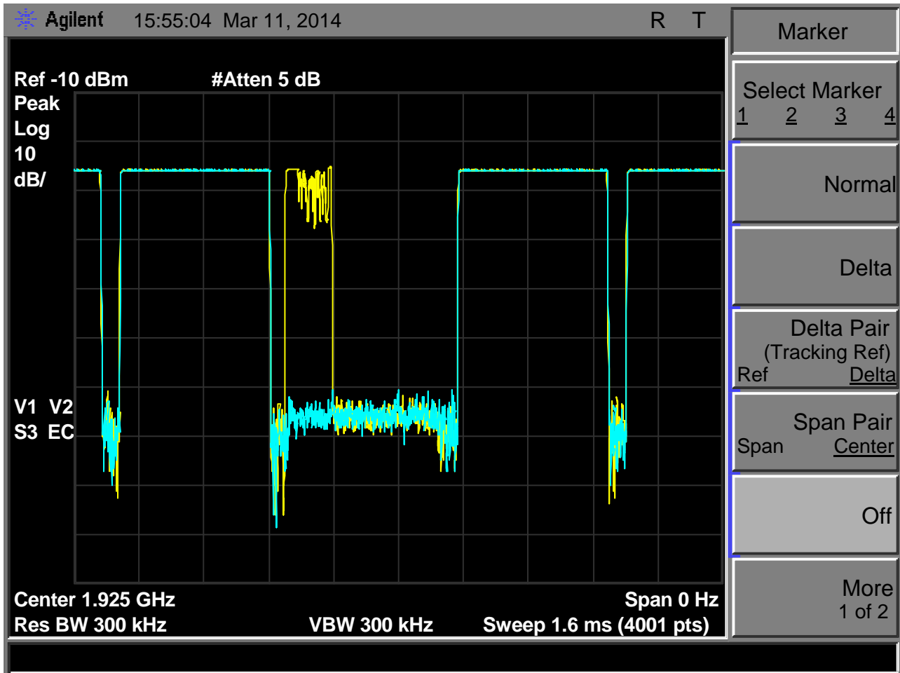
Fig. 68 - Zero-span (single frequency receiver mode) sweep of TDMA interference on carrier at 1924.992MHz, f_1 , with base EUT transmission in single open timeslot, detail of open timeslot and transmission.
