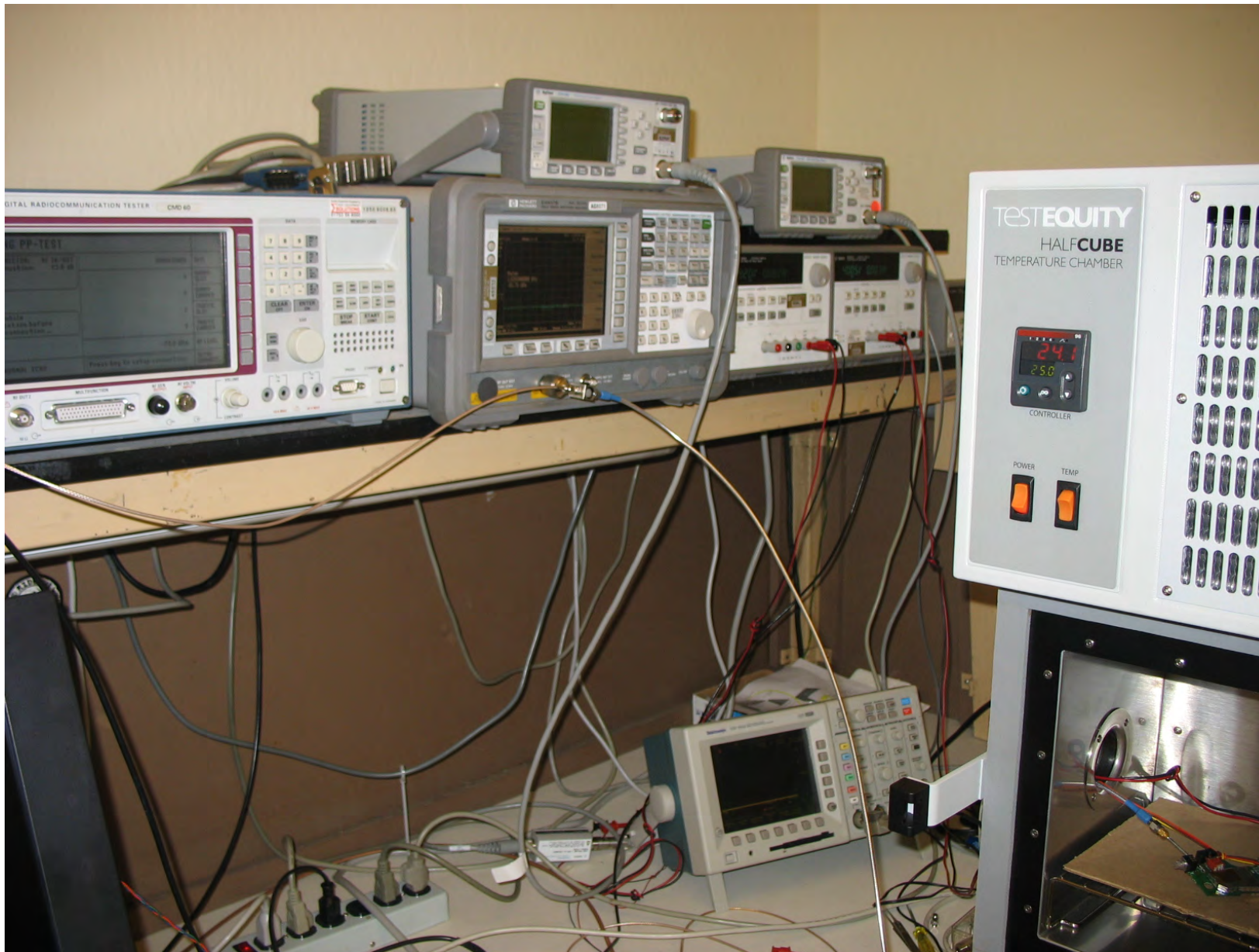
Fig. 110 - View of test system configured for the tests of clause 6.2.1 for the headset EUT. EUT is in the temperature chamber at right. EUT power supply is top right. EUT RF cabling is connected as described in the text, to the CMD60 analyzer and the E4407B spectrum analyzer. The controller interface circuit (RS232 to CMOS levels) is directly outside the chamber egress.
