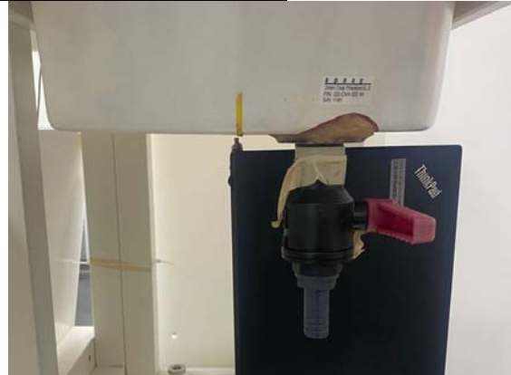
Fig.6 EUT Tip_without cable side to flat phantom
