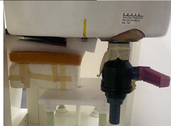
Fig.3 EUT Horizontal-Down side to flat phantom
