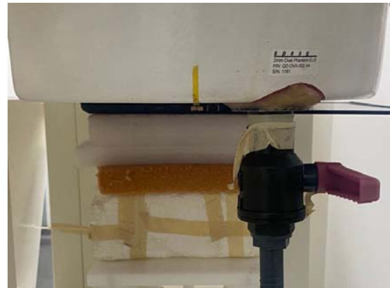
Fig.4 EUT Horizontal-Up side to flat phantom
