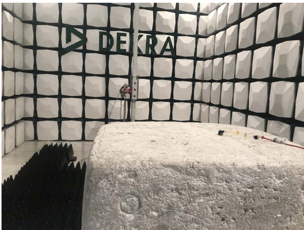
Description: Radiated Emission Test Setup for 1~18GHz
