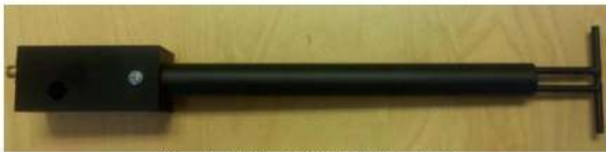
Figure 1 – MVG COMOSAR Validation Dipole
