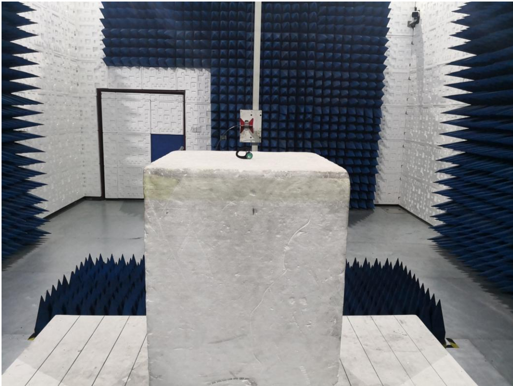
RADIATED EMISSION TEST SETUP ABOVE 1GHZ
