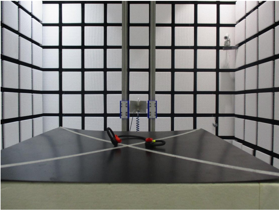
Radiated Emission Test below 1GHz
