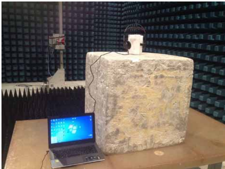
Description: Radiated Emission Test Setup for 1~18GHz
