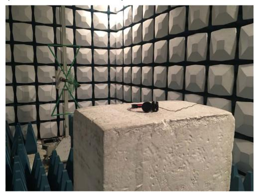
Description: Radiated Emission Test Setup for 1~18GHz
