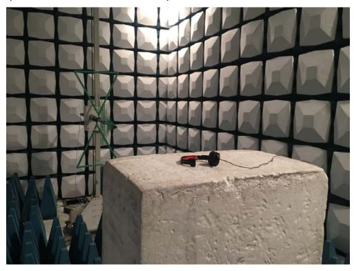
Description: Radiated Emission Test Setup for 1~18GHz
