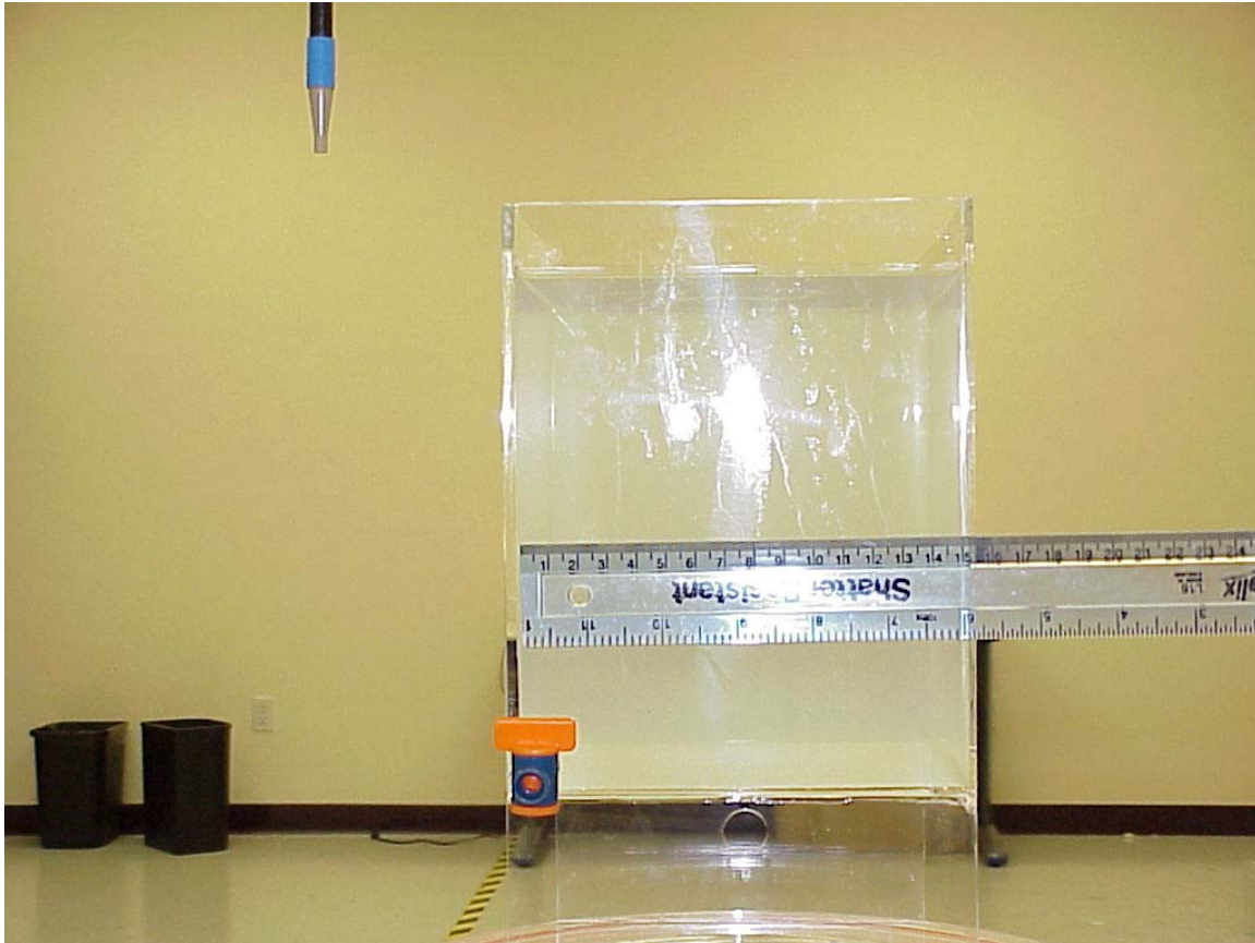
Photo 8: Photo to demonstrate 15 cm Z-axis flat phantom.
