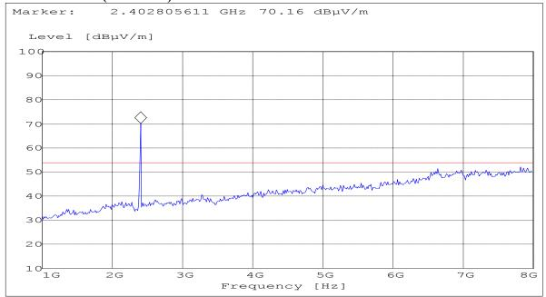
NOTE: The peak above the limit is the carrier frequency.
