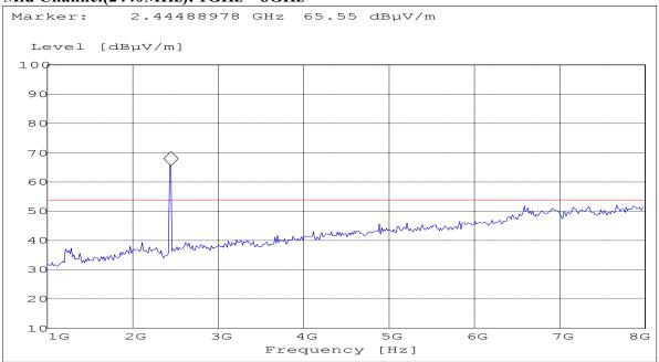
NOTE: The peak above the limit is the carrier frequency. ANALYZER SETTINGS: RBW = 1MHz VBW = 1MHz
