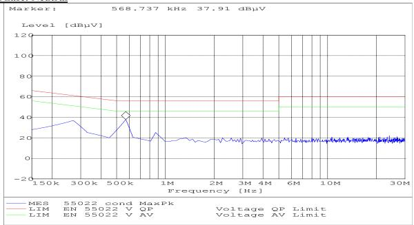
For the AC line conduction tests shown above a dual charger was used with both the headset M1000 and adapter M500 connected. Both units were transmitting and drawing maximum current from the charger.
