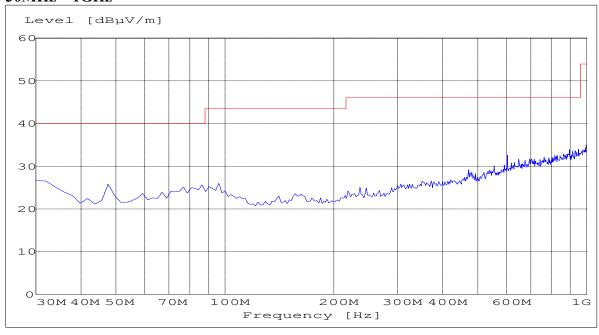
ANALYZER SETTINGS: RBW = 100KHz VBW = 100KHz
