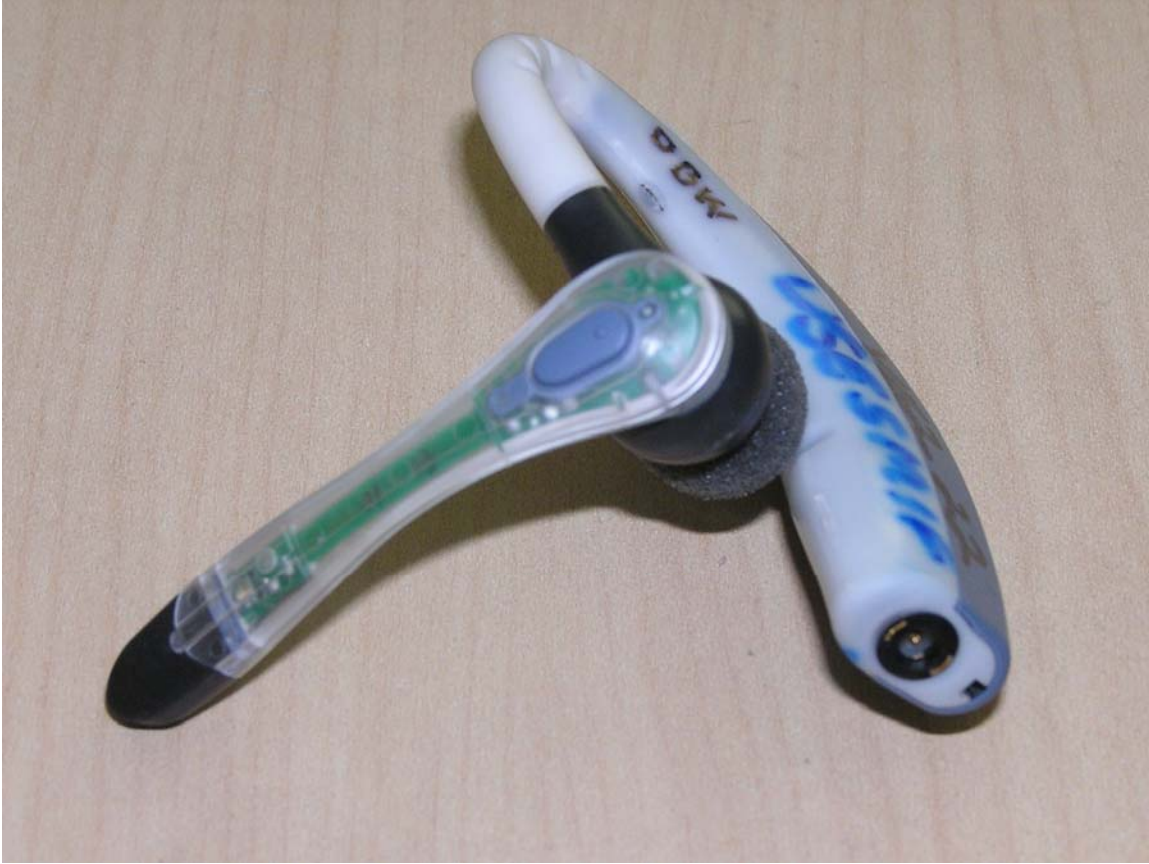
EUT – Profile view showing ac power port
