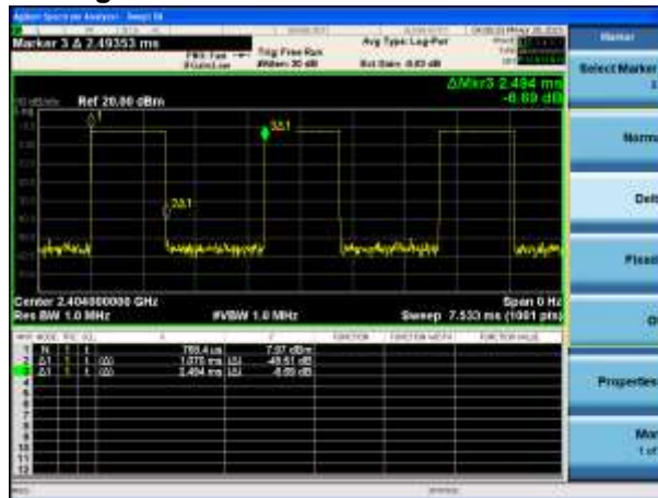
Equation 7-2 Bluetooth LE 2 Mbps Duty Cycle Calculation for Dongle
